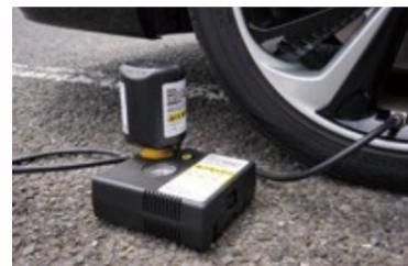
IMS Tire Puncture Emergency Repair Kit
