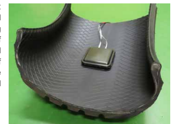
Electricity generation device fitted to the inner surface of a tire
