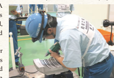
15th Skill Olympics competition (making precise holes in a mold without breaking the drill)
