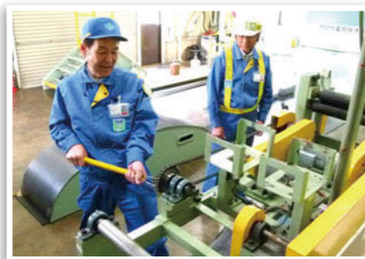
Accident simulation training (Shirakawa Factory: Accident simulation training on getting tangled in a drive chain)
