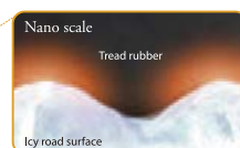
Nanolevel flexibility of rubber helps the tread adhere firmly to irregular icy surfaces.
