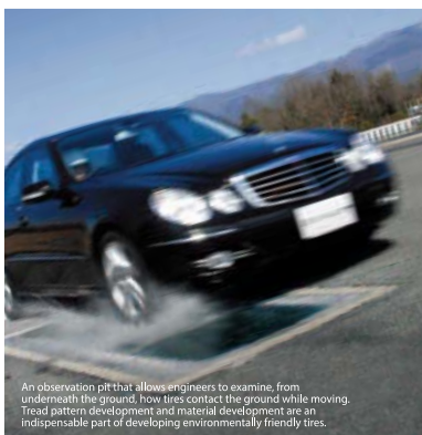
Sumitomo Rubber Tire Technical Center tests rolling resistance and abrasion energy using prototypes.
