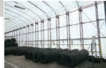
■ The color of tents was changed to white, which made fluorescent lighting unnecessary during the day, resulting in electricity savings. (Ono Factory)
