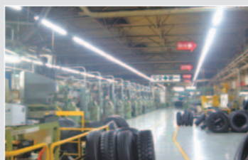
■We've reduced energy consumption for lighting by introducing energy-saving fluorescent lamps in conjunction with the layout change.
